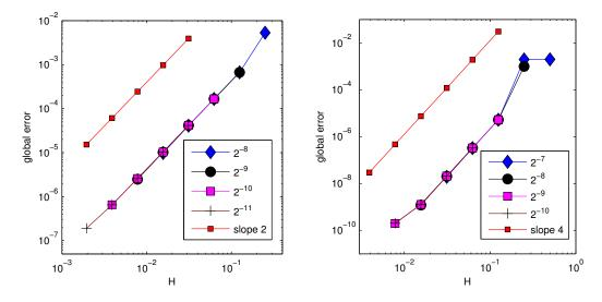
FIGURE 4. Numerical solution of linear test equation (2D) by second-order MRCM combined with Strang splitting method (left) and fourth-order MRCM combined with splitting method by Yoshida (right), respectively, applied with stepsize  $h = T_0 \cdot 10^{-3}$ . Global errors versus increments H for  $\varepsilon = 2^{-8-j}$  with  $j \in \{0, 1, 2, 3\}$  or  $\varepsilon = 2^{-7-j}$  with  $j \in \{0, 1, 2, 3\}$ , respectively. Reference lines of slopes 2 and 4 are drawn correspondingly.
